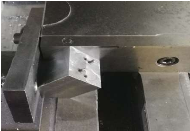
Figure 7. Jig implemented to the production process
